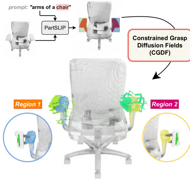
Figure 3.1: CGDF: Constrained Grasp Diffusion Fields produces dense grasp configurations on large, geometrically complex objects (e.g., chairs) in a dual-arm setting. Given target regions (optionally obtained via text prompts using PartSLIP [50]), CGDF employs a part-guided diffusion strategy to efficiently generate grasps localized to these regions, enabling coordinated multi-region and multi-arm grasping.
